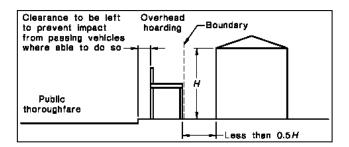
The Principal Contractor must ensure that overhead protective structures are installed and maintained in accordance with the NSW "Code of Practice - Overhead Protective Structures 1995". This is code available at
